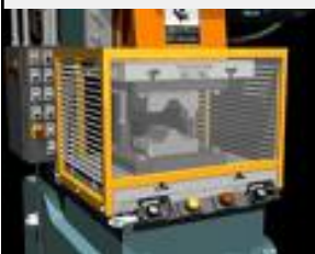
Barrier devices create a safety buffer for employees
