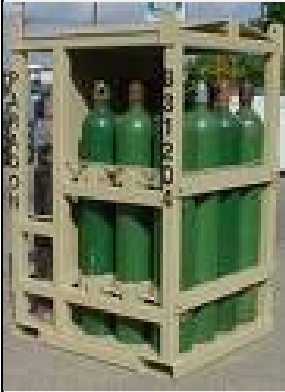
Storage: Cylinders must be secured to prevent tipping.
