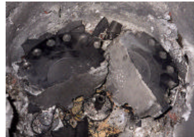
Centrifuge failure, likely due to metal fatigue. (Courtesy of C. Whitaker, MIT)
